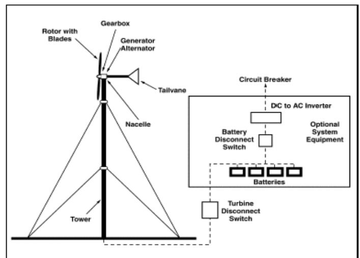
Fig. 2: Components of a wind energy system. (Source: Natural Resources Canada)
