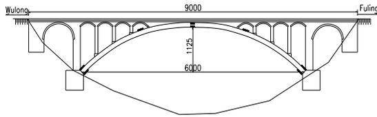
**Fig.6. The layout of vibrating wire sensors**
