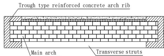
Fig. 3. Trough type reinforced concrete arch rib.
