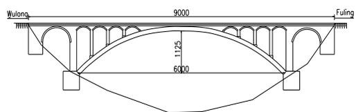
**Fig. 1. The layout of DaXiHe No. 3 bridge (unit: mm).**
