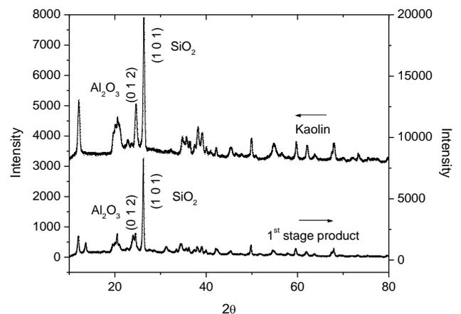
Fig. 3 XRD patterns of kaolin and desilicated kaolin
