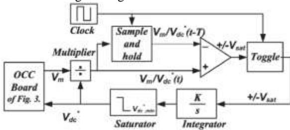
Fig. 5. block diagram of mppt realization
