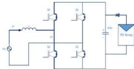
Fig.2 1Ø single stage grid connected pv system
