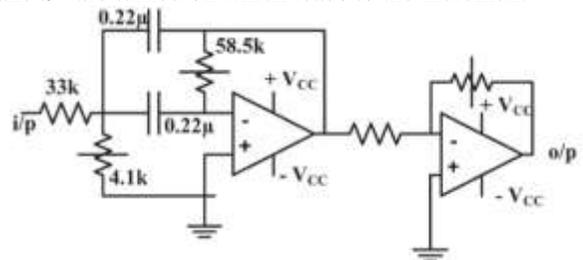
Fig. 4-Circuit diagram of analog implimantion of BPF
