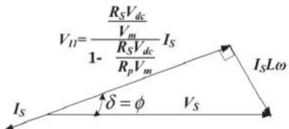
Fig.5-Phasor diagram depicting the steady-state comporment of the proposed voltage-sensor less system.
