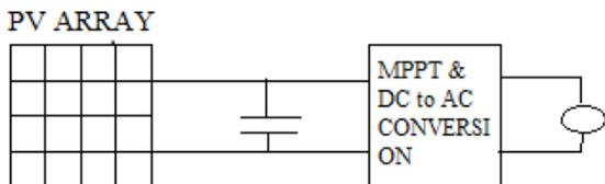
Fig.1 A generic grid connected PV system.
