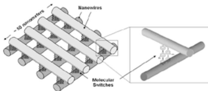
Fig.1 molecular scale crossbar ckt architecture
