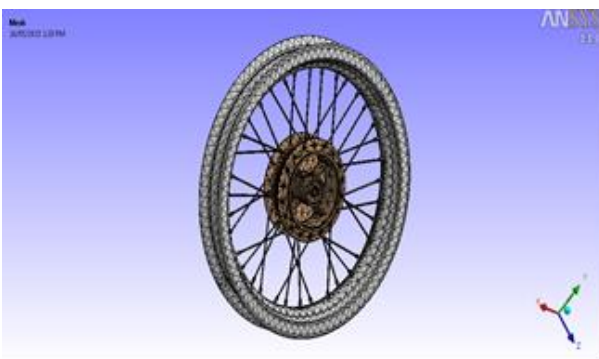
Fig. 8. Meshed model of Existing wheel.
