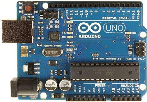
Fig. 5 Arduino board
