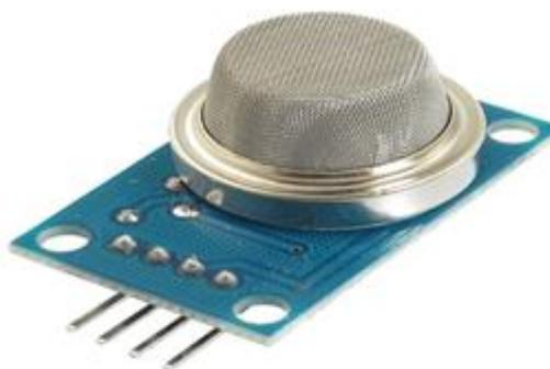
Fig. 3 Alcohol sensor
