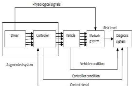
Fig. Controller based drowsiness detection system
