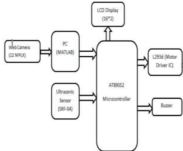
Fig. Block diagram of overall system
