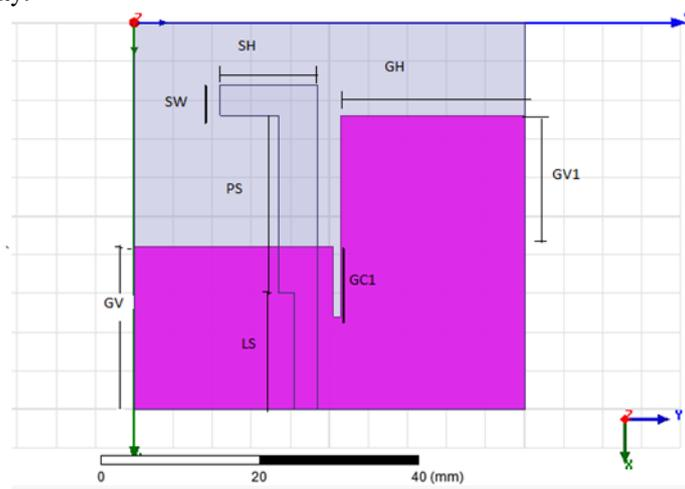
Fig 1: Structure of proposed Microstrip antenna type(A).
