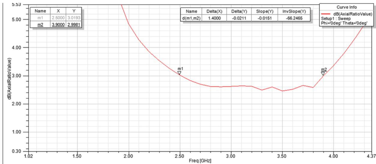
Fig 2: Graph of Axial ratio of MSA type(A).
