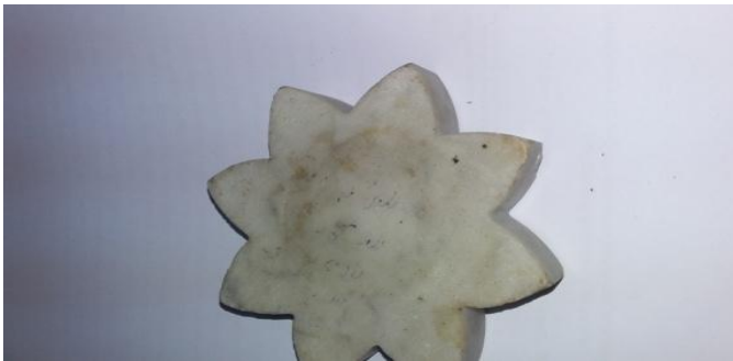
Fig. 10a a toothed disc shaped with water cutting jet using MF garnet particles
