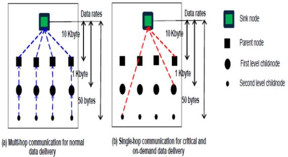
Fig. 7. Energy management for single-hop and multi-hop communication
