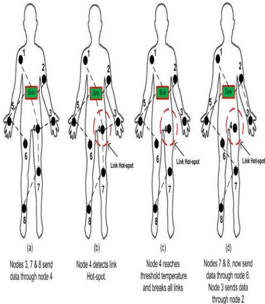
Fig. 6. Link Hot-spot detection
