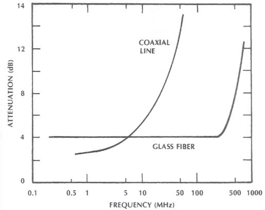
**Figure 4:** Effective attenuation of a 1 km length of coaxial line and glass fiber. The 3 dB bandwidth of the fiber is 500 MHz [8]
