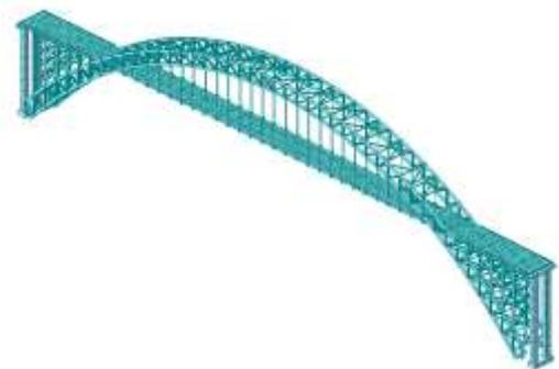
Fig. 2 The spatial finite element model of the Yangtze River Highway Bridge
