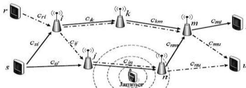
Fig. 1: An example network with sources  $S = \{r, s\}$  is illustrated. Each unicast link  $(i, j) \in E$  is labeled with the corresponding link capacity.
