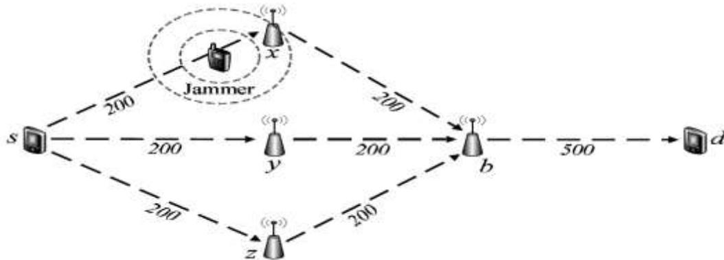
Fig. 2. Illustrates a single-source network with three routing paths.
