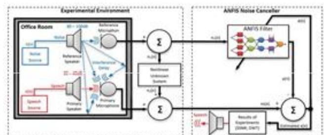
Figure 2: Simplified Principal Scheme of Adaptive Noise Suppression in Voice Communication Using the Neuro- Fuzzy Inference System.
