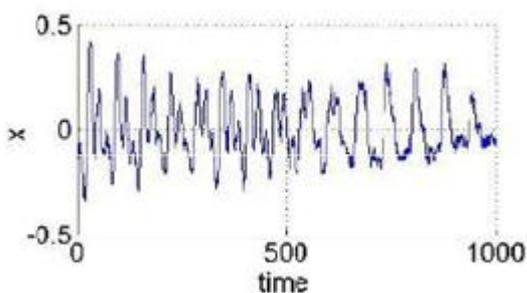
The interference signal which is generated with the non linear characteristic of noise is shown in figure6. This signal is used as second input with m signal contains signal and noise as first input for the system.
