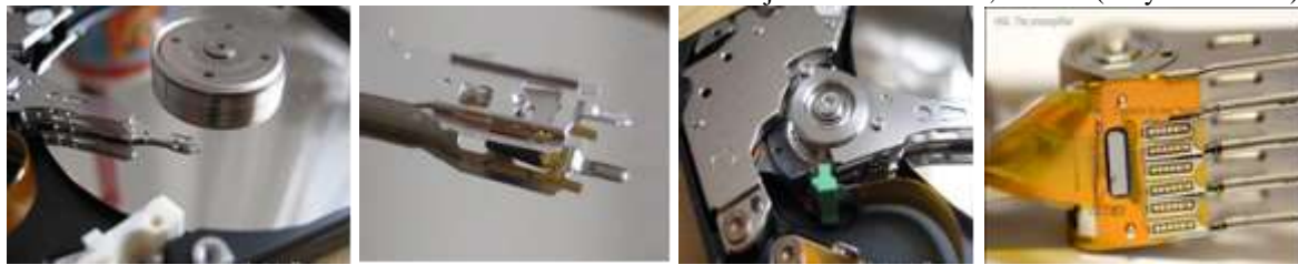
Figure 9: Read & Write Head of HDD
