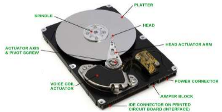
Figure 3: Diagram labelling the major components of a HDD
