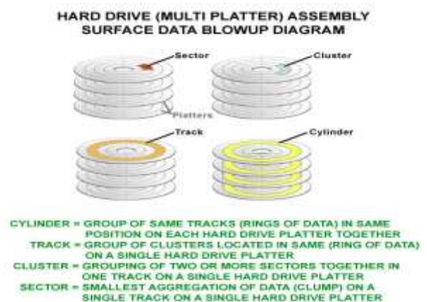
Figure 10: Multi Platter Surface of HDD
