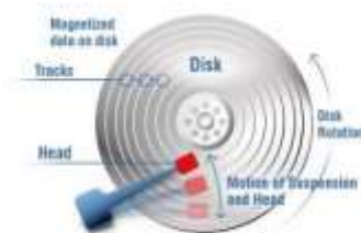
Figure 8: HDD operation motion
