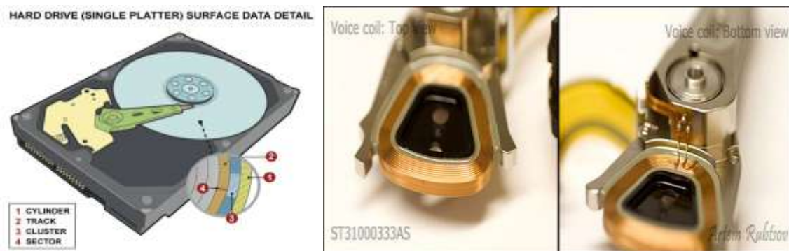
Figure 10: Single platter surface of HDD and Voice Coil
