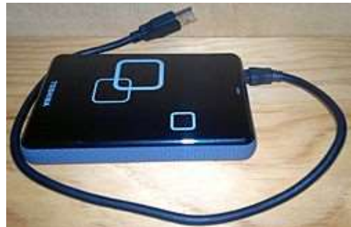
Figure 14: Toshiba 1 TB 2.5" external USB 2.0 HDD
