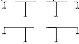
**Fig 1. First side span than middle Schematic diagram**
