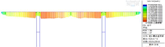
Fig5 Scheme I main girder roof stress diagram
