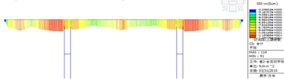
Fig8 Scheme II main girder floor stress diagram
