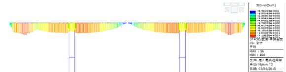
**Fig19 Scheme I main girder floor stress diagram**
