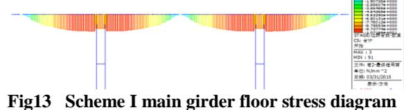
Fig13 Scheme I main girder floor stress diagram
