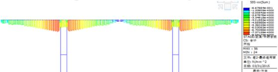
**Fig17 Scheme I main girder roof stress diagram**
