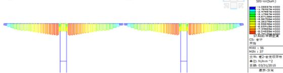
**Fig18 Scheme II main girder roof stress diagram**
