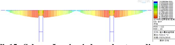
**Fig15 Scheme I main girder webs stress diagram**
