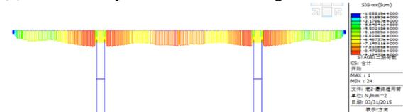
Fig9 Scheme I main girder webs stress diagram
