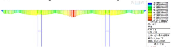
Fig7 Scheme I main girder floor stress diagram
