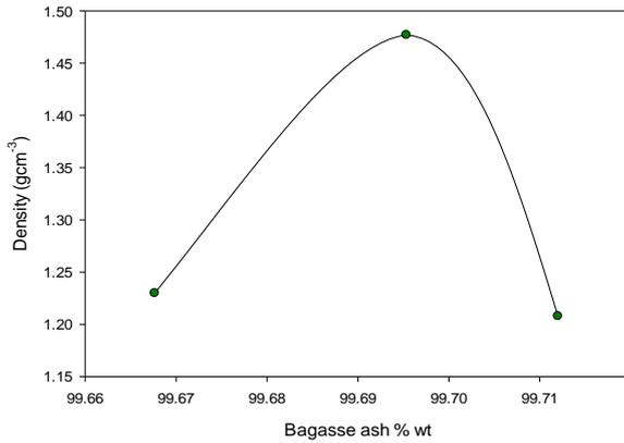
Fig. 9 Density versus the weight of Bagasse Ash
