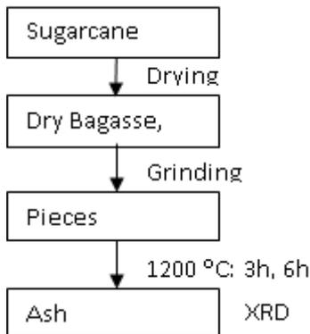
Fig. 5(a) Schematic representation of bagasse ash
