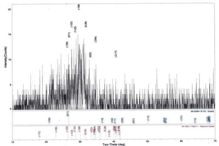
Fig.6 (b) XRD pattern of Bagasse ash at 1200°C for 6h
