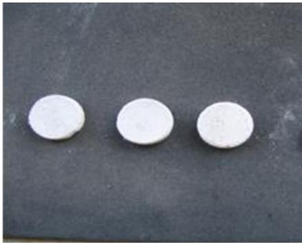
Fig. 4 .The photograph of Bagasse Ash specimens
