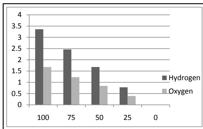
Fig. 1. Gas Production (L) v Battery Charge (%). Y-axis shows amount in liters and x axis shows battery charge percentage
