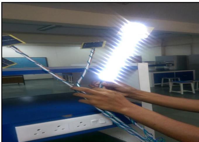
Fig. 1. LED Lights in on state when light intensity dropped below 100lux
