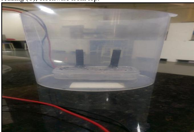
Fig. 1. Electrolysis jar containing two graphite (carbon) electrodes
