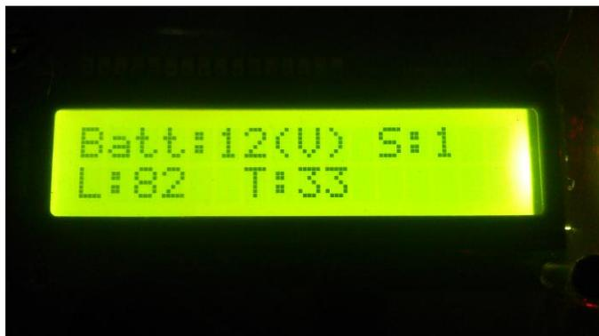
Fig. 2. LCD Screen showing battery voltage (Batt), timer (S), light intensity (L) and thermistor reading (T), clockwise from top
