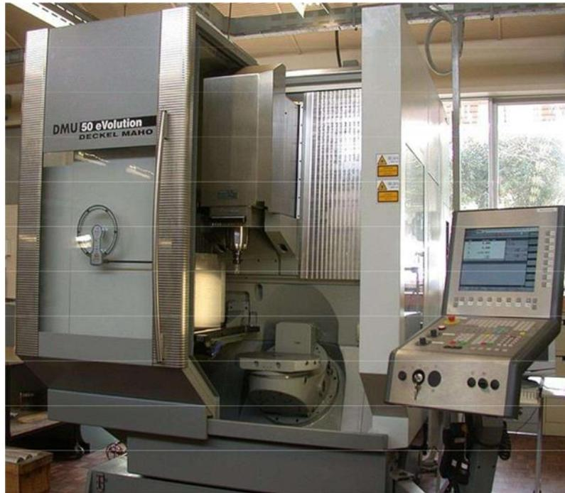
Figure 3. 1 CNC Milling machine
