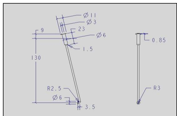
**Fig.3. Geometric model of Spoke.**
