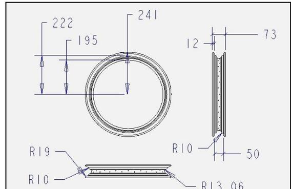
**Fig.1. Geometric model of existing rim.**
