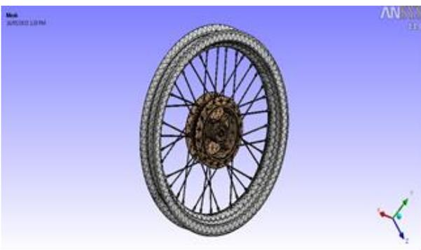
Fig. 8. Meshed model of Existing wheel.
