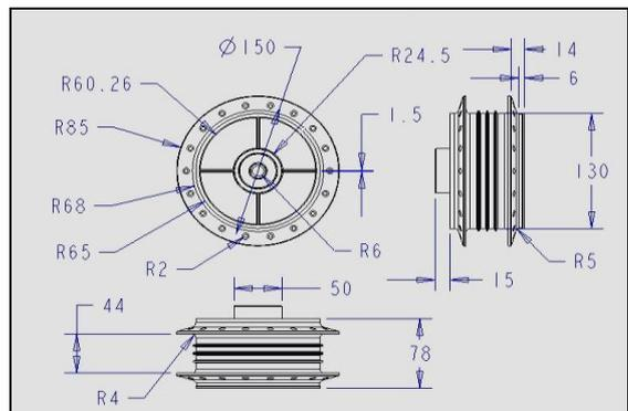
**Fig.2. Geometric model of Hub.**
