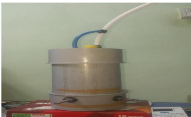
Fig.3. Photo electro chemical cell
