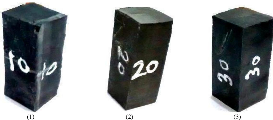
Figure 3.3: Specimens for Compressive Test
