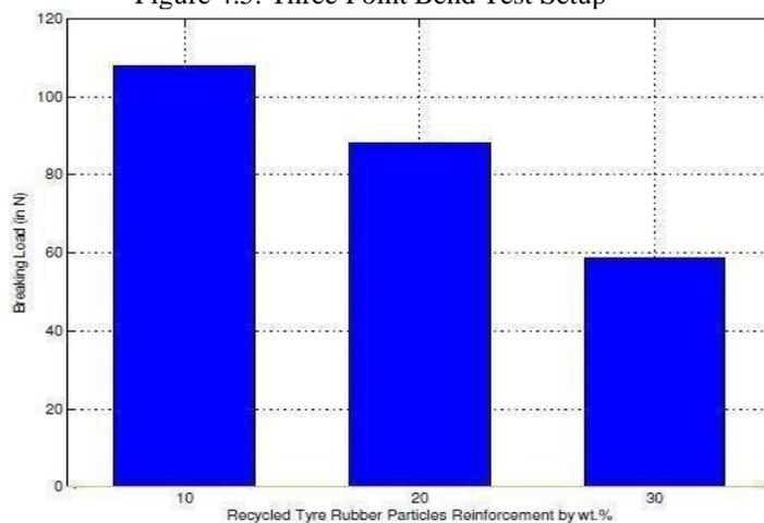
Figure 4.6: Flexural Load at break with variation of tyre rubber particles reinforcement by wt. percentage
