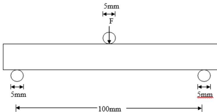
Figure 4.5: Three Point Bend Test Setup
