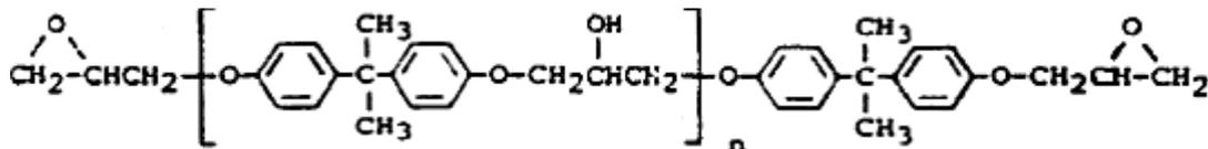
Epoxy application resins are widely: adhesives, bonding, building materials (flooring, paving and aggregates), composites, laminates, coatings, molding, and textile finishing. He has recently found use in the air- and spacecraft industries.
