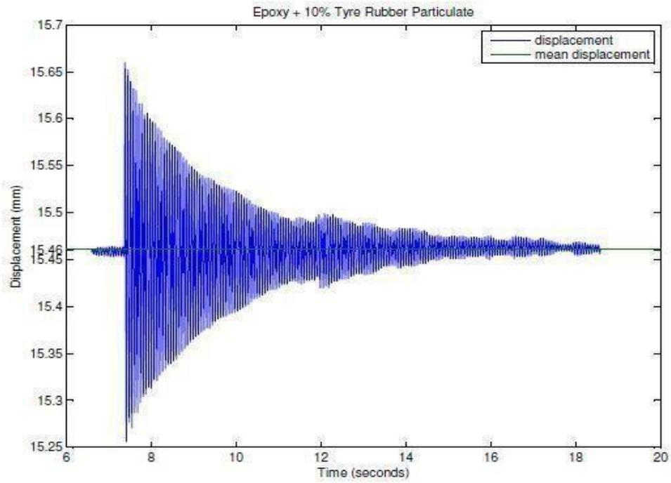
Figure 4.9: Time domain response of Epoxy + 10% (by wt.) Tyre Rubber particulate beam
