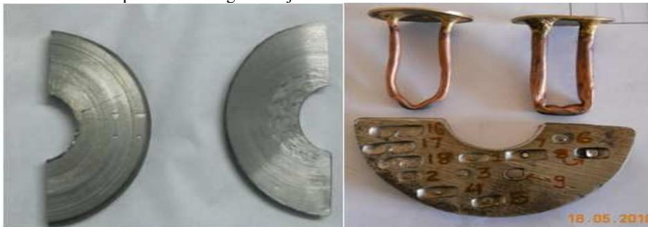
**Figure 3.4 P-20 workpiece before and after machining with tool**
