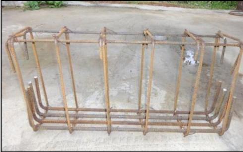
Fig. 1. Reinforcement cage for deep beam
