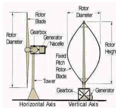
Figure 2.3: Comparison of HAWT and VAWT
