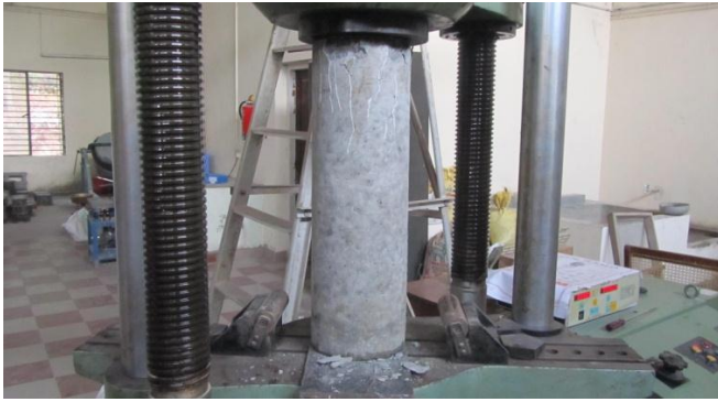
Fig: 4. Compression testing of column
