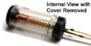
Fig6: Internal structure of vibration sensor
