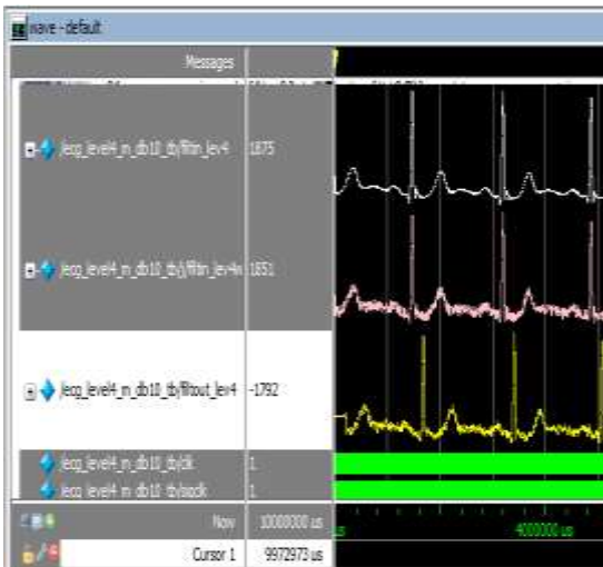
Figure 8: Noise free ECG waveform at output, after noise being added to it.
