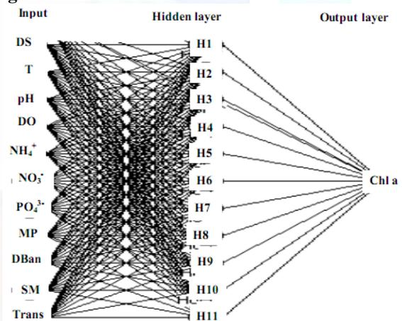
Fig. 3. Architectural network of model 11-11-1
