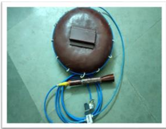
Figure 2. Final arrangement of the jack.
