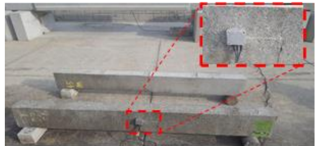
Fig.10: Vibration test of Plain concrete beams
