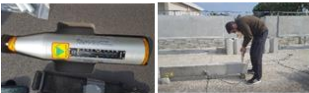
Fig.5. Schmidt R Hammer and compressive strength testing
