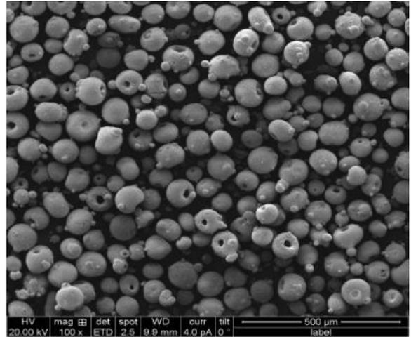
Figure 5: SEM image of  $\text{ZrO}_2$  powders at 200x magnification.
