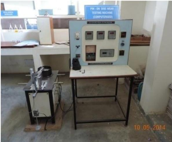
Figure 3: Wear testing machine
