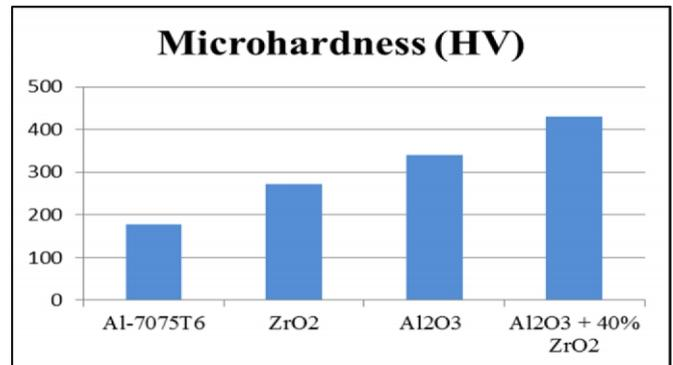
Figure 10: Micro-hardness of uncoated and coated specimen
