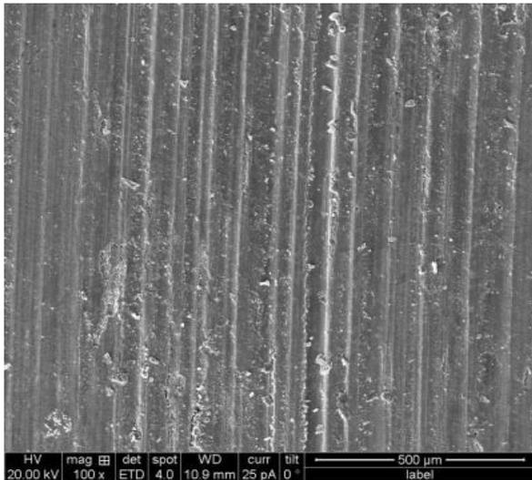
Figure 17: SEM of Al-7075T6 specimens after wear test.
