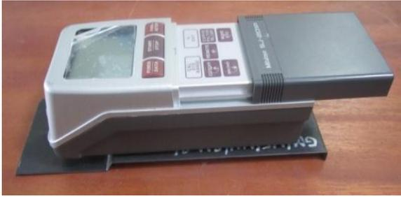
Figure 2: Talysurf (Surface roughness tester Model: SJ-301)
