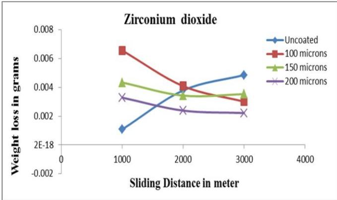
Figure 12: Effect of sliding distance on wear loss for  $ZrO_2$
