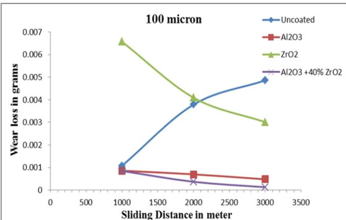
Figure 14: Effect of sliding distance on wear loss for a 100  $\mu m$
