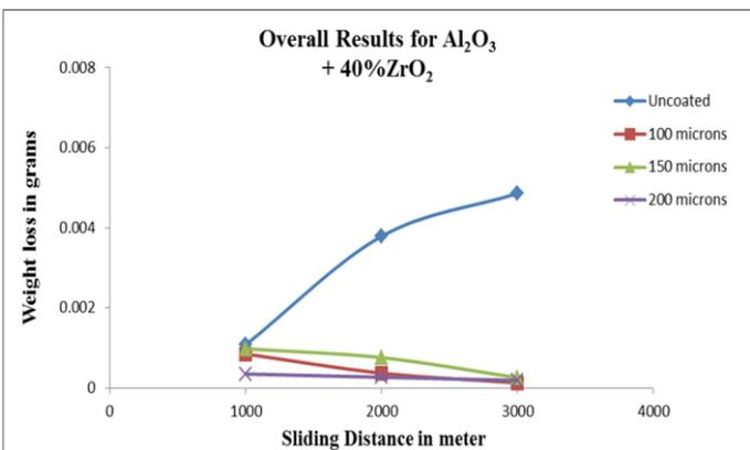
Figure 13: Effect of sliding distance on wear loss for  $Al_2O_3 + 40\% ZrO_2$
