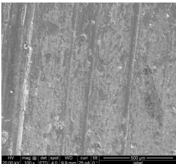
Figure 19: SEM of ZrO<sub>2</sub> coated specimens after wear test.
