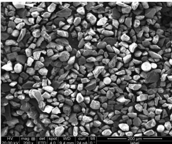
Figure 4: SEM image of  $\text{Al}_2\text{O}_3$
