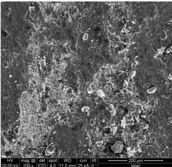
Figure 18: SEM of Al<sub>2</sub>O<sub>3</sub> coated specimens after wear test.
