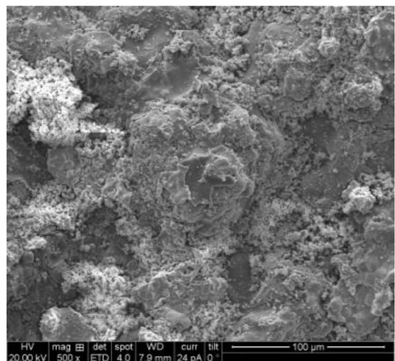
Figure 7: SEM image of  $\text{ZrO}_2$  coated specimen
