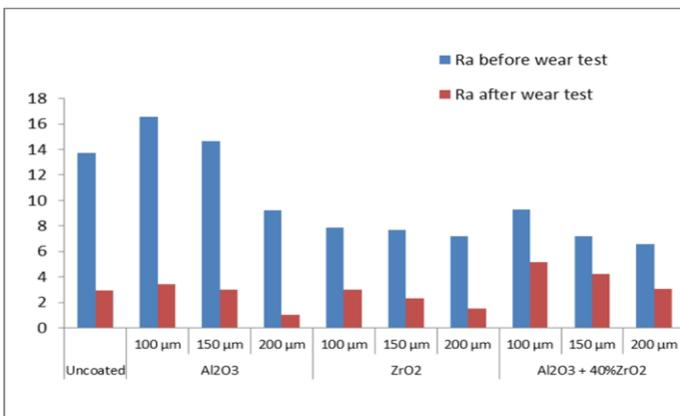
Figure 9: Surface Roughness of uncoated and coated specimens
