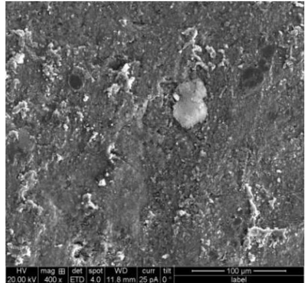
Figure 20: SEM of Al<sub>2</sub>O<sub>3</sub> + 40% ZrO<sub>2</sub> coated specimens after wear test.
