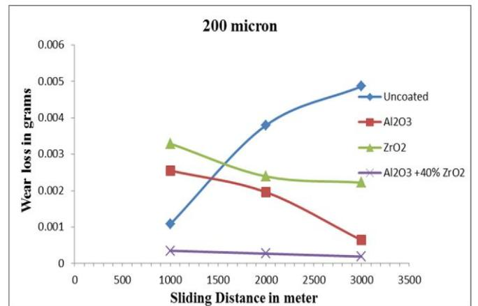
Figure 16: Effect of sliding distance on wear loss for 200  $\mu m$
