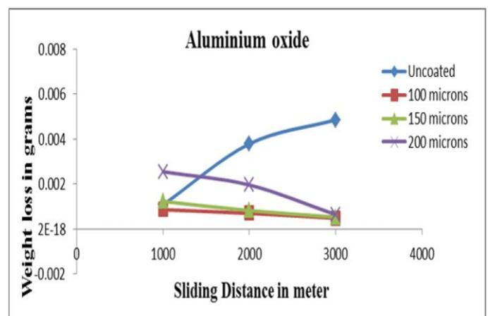
Figure 11: Effect of sliding distance on wear loss for Al<sub>2</sub>O<sub>3</sub>
