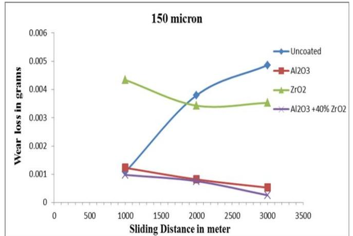
Figure 15: Effect of sliding distance on wear loss for 150  $\mu m$
