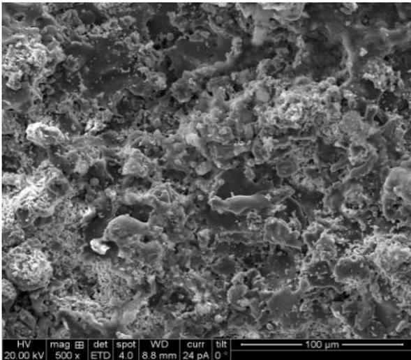
Figure 8: SEM image of Al<sub>2</sub>O<sub>3</sub>+40%ZrO<sub>2</sub> coated specimens
