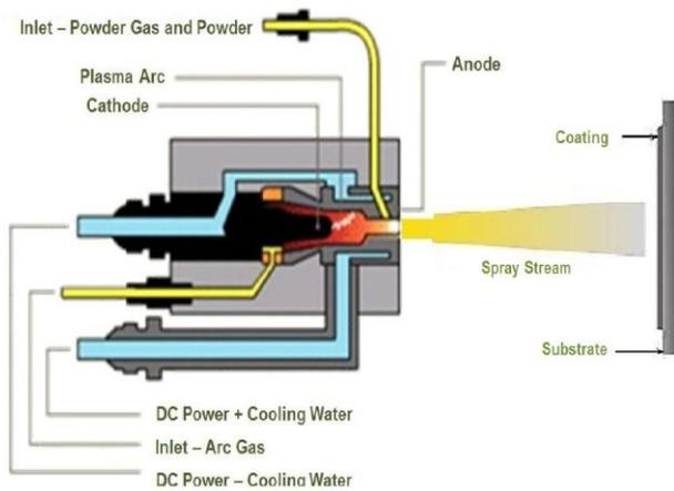
Figure 1: Plasma-Arc Gun Cross section
