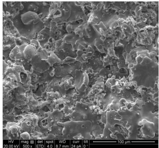
Figure 6: SEM image of  $\text{Al}_2\text{O}_3$  coated specimen.
