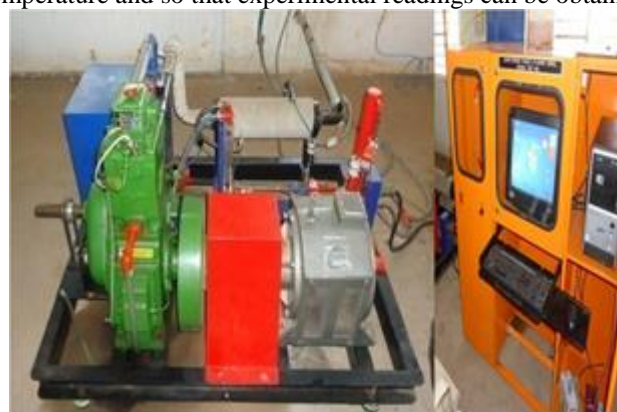
Figure4: Single cylinder 4-stroke CI engine with computerized control panel
