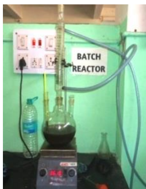
Figure2: batch reactor (3-neck flask)
