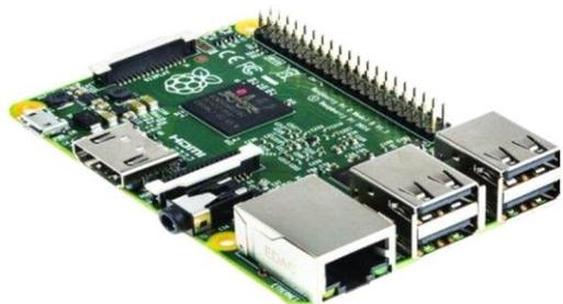
Fig1:Raspberrypi (model 2B)
