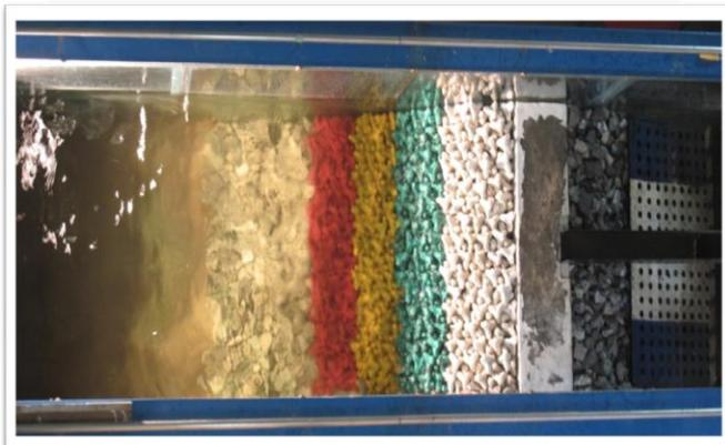
**Figure 4 Overtopping chute and container**
