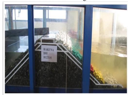
Figure 3. Model cross-section as built
