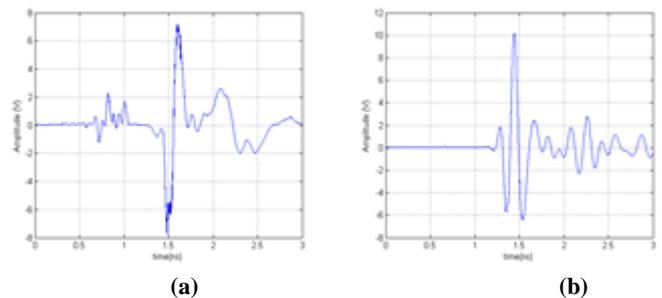
Fig. 2. (a) Waveform of the generated pulse by generator head, (b) Waveform of radiated pulse by antenna
