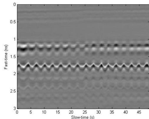
Fig. 4. Signal with Background Clutter Removed
