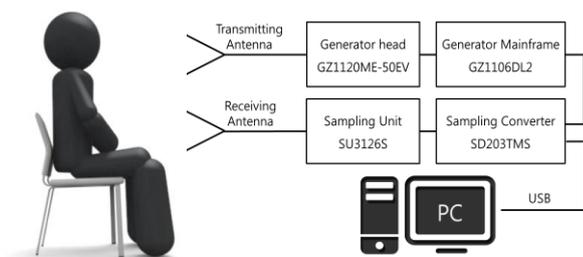
Fig. 1. UWB Measurement Schema
