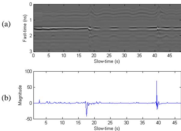
Fig. 6. (a) Received Raw Data, (b) Movement Signal after Operating Detection Algorithm
