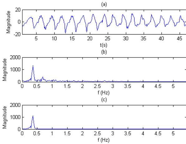
Fig. 5. (a) Respiration Signal, (b) FFT of Noisy Signal, (c) FFT of Filtered Signal
