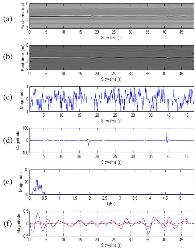
Fig. 7. (a) Raw Data, (b) Signal after Clutter Removal, (c) Respiration Signal in Time Domain, (d) Movement Signal in Time Domain, (e) FFT of Filtered Signal, (f) Filtered Respiration Signal in Time Domain (blue), and CFAR Threshold (red)
