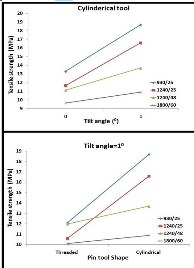
**Fig. 1: Tilt angle and pin tool shape versus tensile strength**
