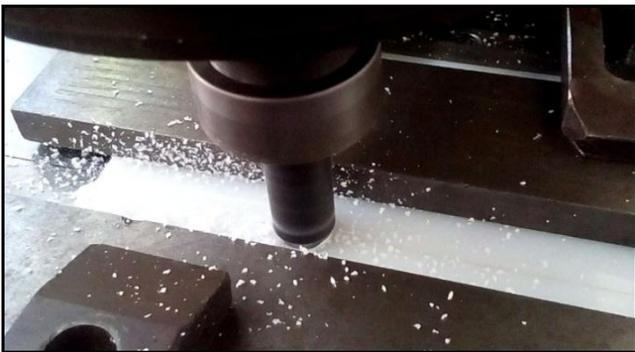
**Fig. 12: High rotation speed caused ejection of polymer**
