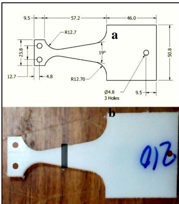
**Fig. 9: Fatigue specimen [30]**
