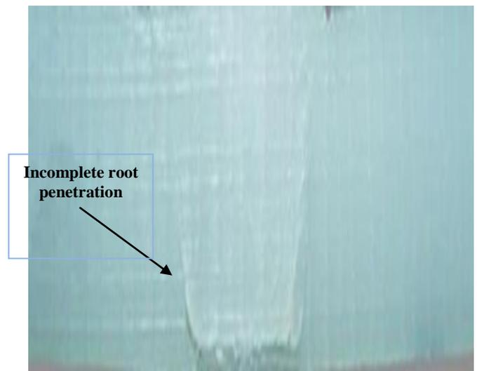
**Fig. 16: Incomplete root penetration weld defect**
