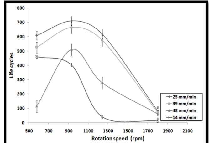
**Fig. 15: Effect of rotation speed on fatigue life at different travel speeds**
