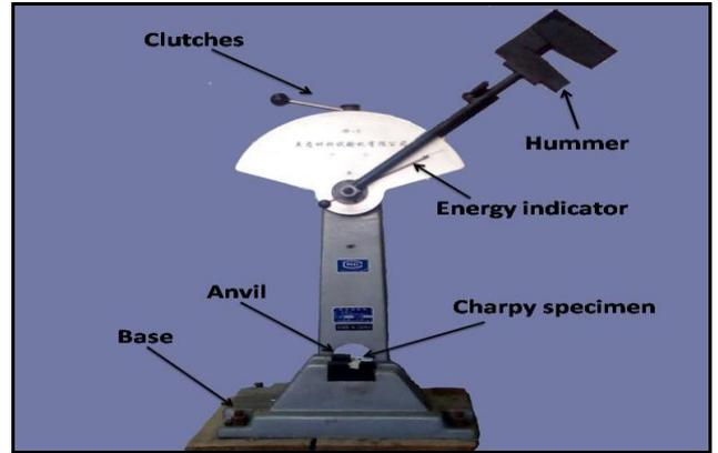
**Fig. 6: Impact-testing machine**
