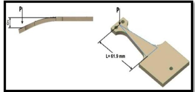
**Fig. 10: Design of fatigue taper cantilever specimen [31]**
