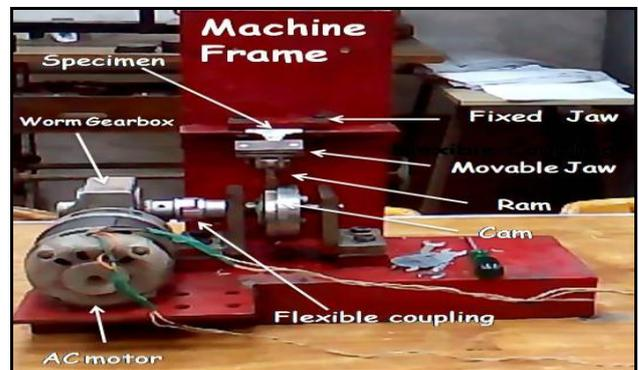
**Fig. 7: Reciprocating fatigue bending testing machine**
