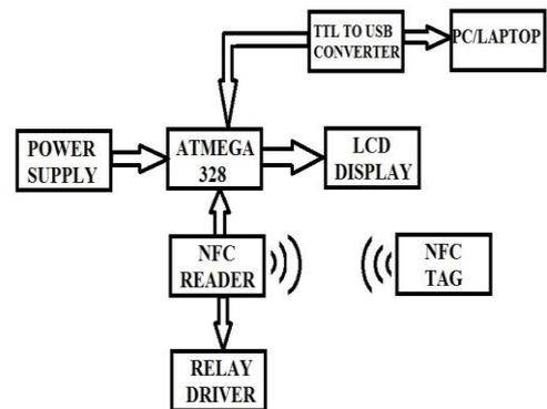
Figure 4: NFC Block Diagram.
