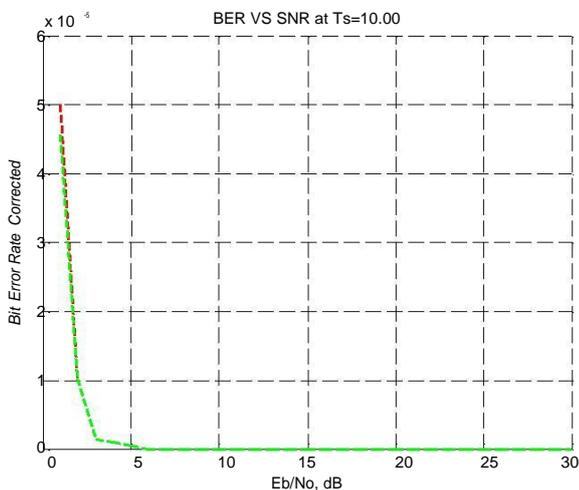
Fig7. BER vs SNR graph for Rician channel with constant Ts
