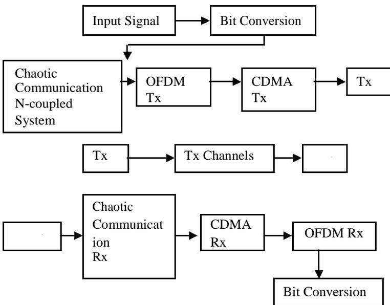
Figure 3 Block diagram of proposed transmission system
