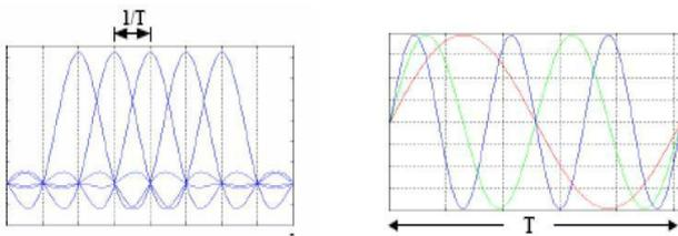
Figure 1 frequency spectrum of an OFDM transmission
