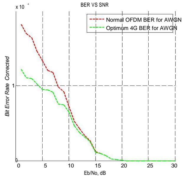
Fig 4: BER vs SNR graph for AWGN channel
