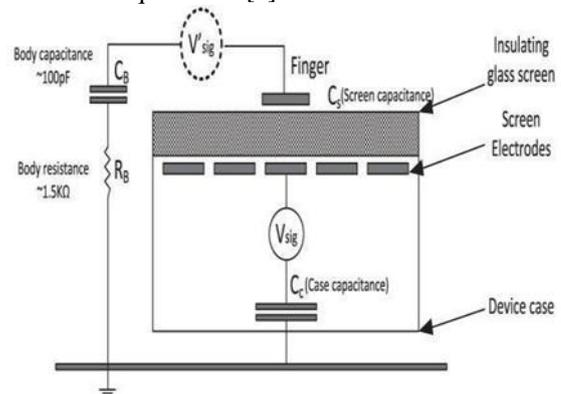
Figure 3.schematic of a basic capacitive touchscreen
