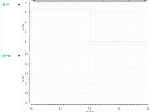
Figure 4: Waveform of a CMOS Inverter with LECTOR.
