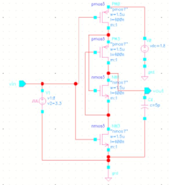
Figure 3: CMOS Inverter with LECTOR
