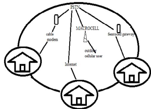
**Fig 1: cross tier interference between femtocell and macrocell**
