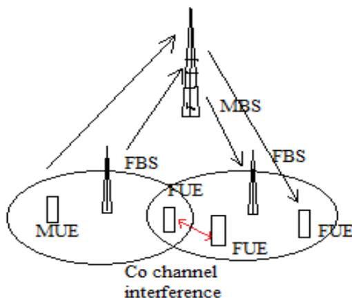
Fig.2 Downlink Interference in femtocells.
