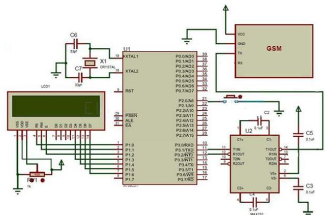
Fig5.Interfacing of 89c51 with GSM Module
