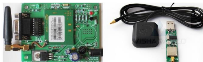
Fig. 3. SIM300 and EB-3531 with external antenna
