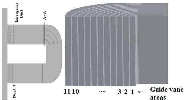
Figure 3. The guide vane (cut view of the guide vane) a) location of A-A cut and b) the areas
