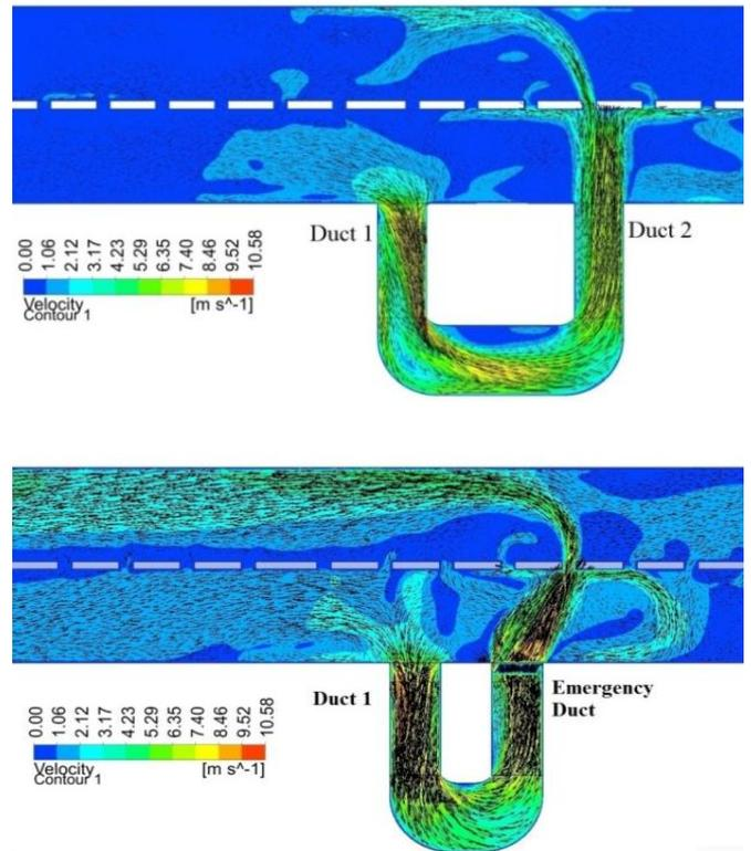
Figure 2. The velocity distributions in the tunnel and the mechanical shafts connected as a) Duct 1&Duct 2 and b) Duct 1&Emergency Duct
