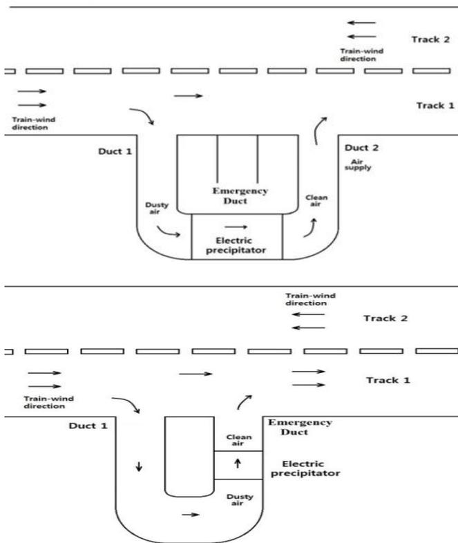
Figure 1. The schematic view of the shafts connections as a) Duct 1&Duct 2 and b) Duct 1&Emergency Duct
