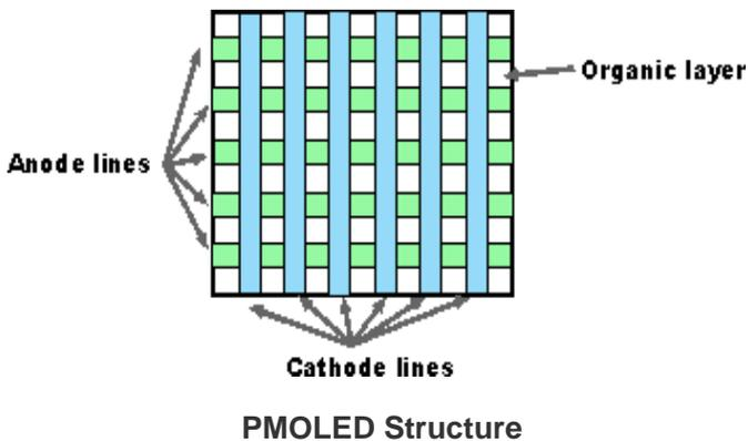
The organic material is set down between the anode and cathode - with both the organic material and cathode metal regions being deposited using relatively standard processes. This enables large scale manufacturing to be achieved in a relatively cheap manner.
