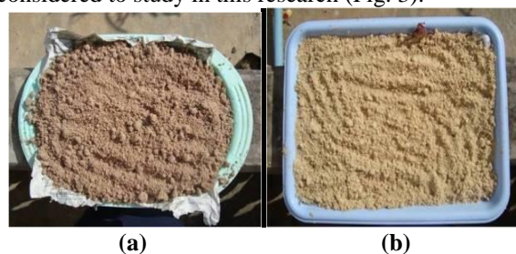
Fig. 3. Raw Substrates after Air Dry at Room Temperature (a) Groundnut Meal Powder (b) Soy Bean Meal Powder
