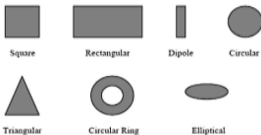
Figure 2.2 Types of Patch Antennas
