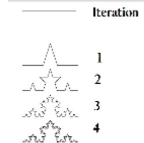
Figure 2.9: Steps of construction for Koch curve geometry
