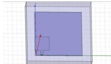
Fig 6. Implemented PIFA antenna
