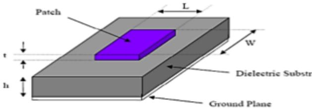
Figure 2.1: Patch Antenna Basics
