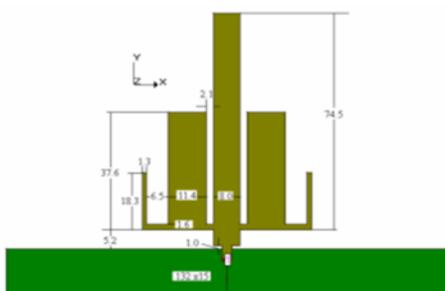
Fig 1. Extended E shape monopole antenna
