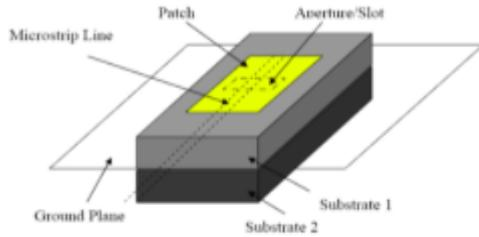
Figure 2.5 Aperture Couple Feed
