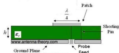
Fig 2. The Planar Inverted-F Antenna (PIFA).
