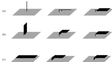
Figure 2.11: Development of PIFA from monopole, planar monopole and microstrip patch antennas.
