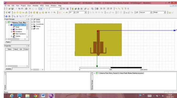
Fig 4.Implemented Monopole structure.
