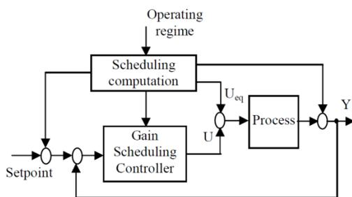
Fig. 3. Control scheme with Gain Scheduling controller type [17]
